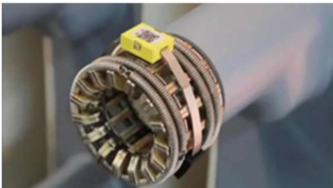
Installed on Moving Contact of Circuit Breaker
